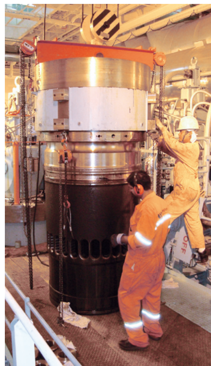
Overhaul of cylinder unit on large bore engine
